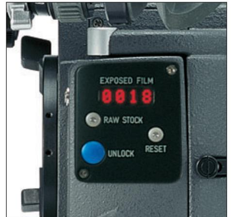
ARRICAM Lite Extended Camera Footage Display
