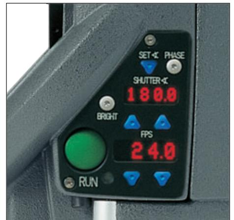
ARRICAM Lite Extended camera control panel
